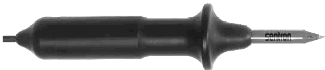
Figure 1. Sentron probe used in pH meter field test. The stabbing portion of the probe is 5 cm in length, with the last 1.7 cm tapering to a sharp point. The sensing membrane is contained in the tapered point.
