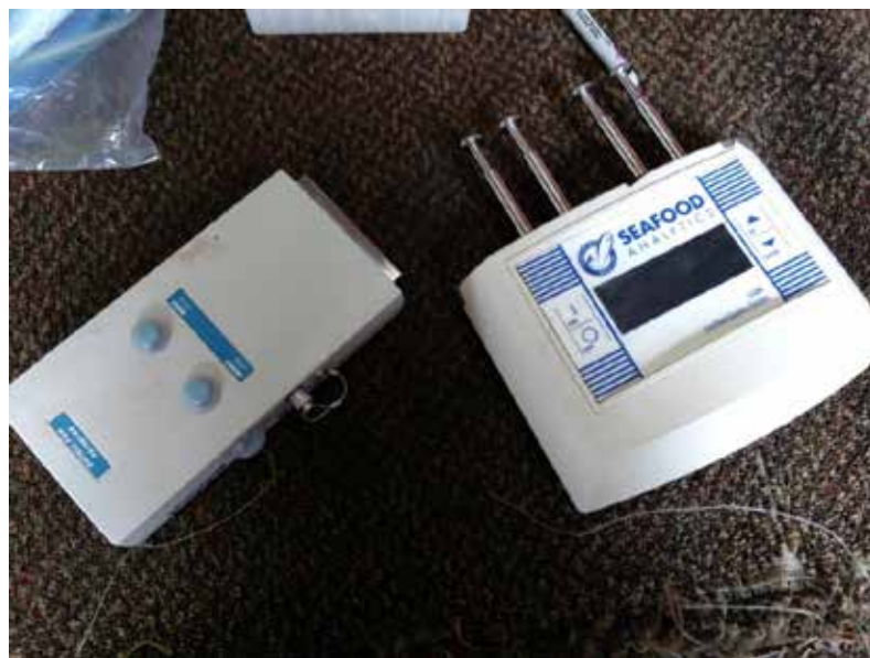
Figure 4. Hand-held device used to estimate somatic fat content using microwave-technology (left) and quality reader used to obtain Phase Angle values (right).
