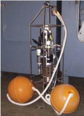
**Missing Profiler One.** A profiler was lost on July 30, 2009 off the east side of Kodiak Island at 56°49.95N latitude and 153°09.12W longitude in about 45 fathoms of water. When lost, the profiling instrument had a 40 pound anchor attached via buoy line and is thought to be sitting hard on-bottom.
