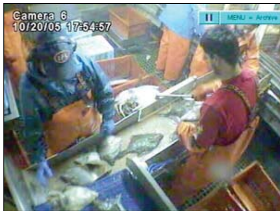
Figure 12. Modified flow scale camera view, showing unsorted catch transferring from the flow scale to the sort conveyor belt at the observer work station (compare with Figure 8f).
