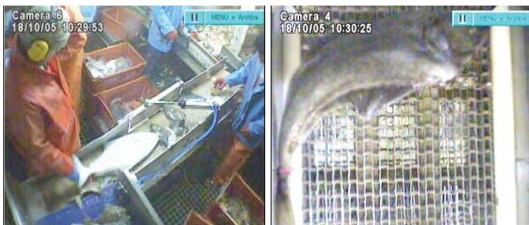
Figure 15. A pink-tagged halibut in the flow scale/ observer station (left), and the same pink-tagged halibut moving up the port discard lift conveyor (right).
