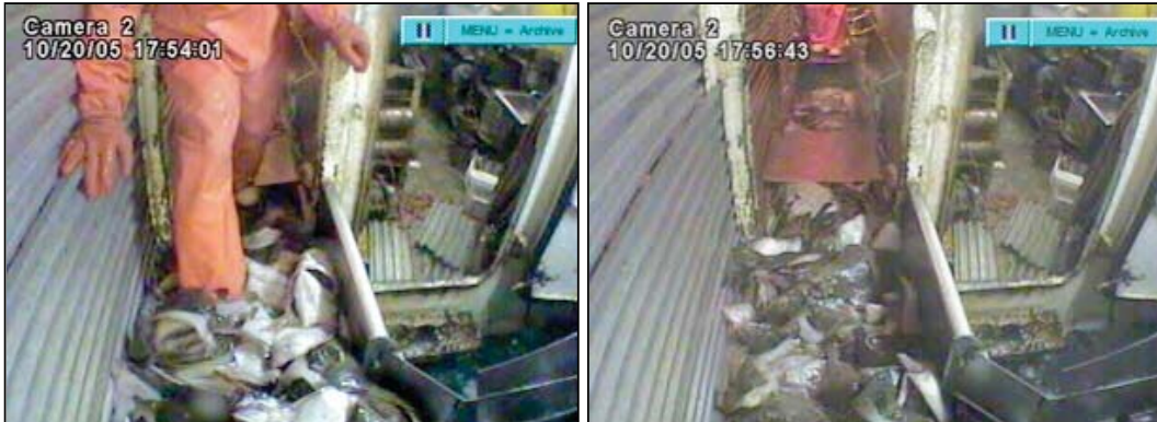
Figure 11. Adjusted fish holding tank camera view, showing kicker feeding unsorted catch onto the first lift conveyor belt (compare with Fig. 8c).
