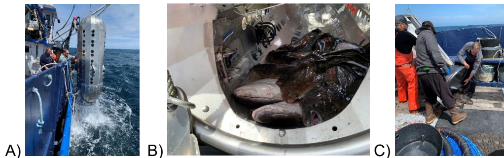
Figure 17. Shuttle being retrieved (A), catch entrained in shuttle (B), and catch being released onto the vessel deck (C).
