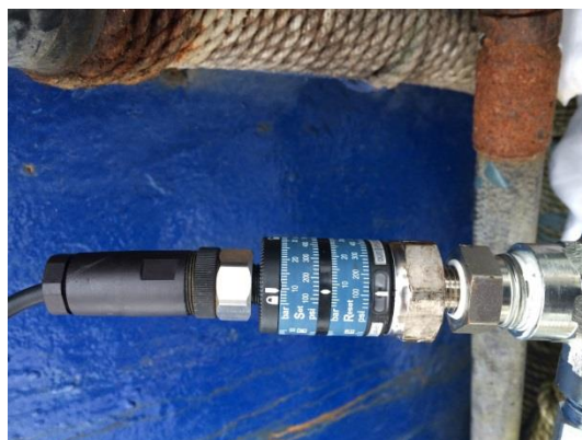
Figure 24a. Image of AMR leads from Hydro sensor 24b. NOAA Fisheries hydro switch sensor installed
