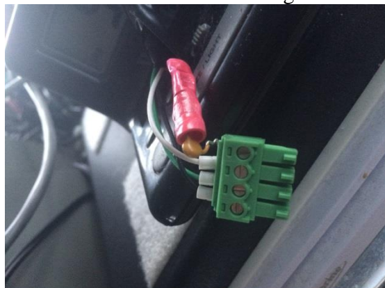
Figure 24a. Image of AMR leads from Hydro sensor 24b. NOAA Fisheries hydro switch sensor installed
