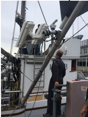
Figure 23a. Cameras set installed on a stabilizer.
