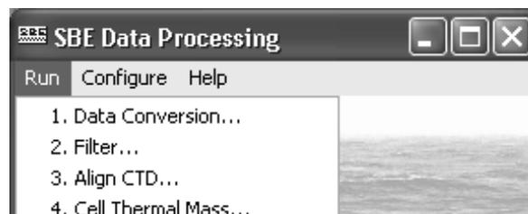
Figure 3.5 Begin converting hex files to cnv files.
