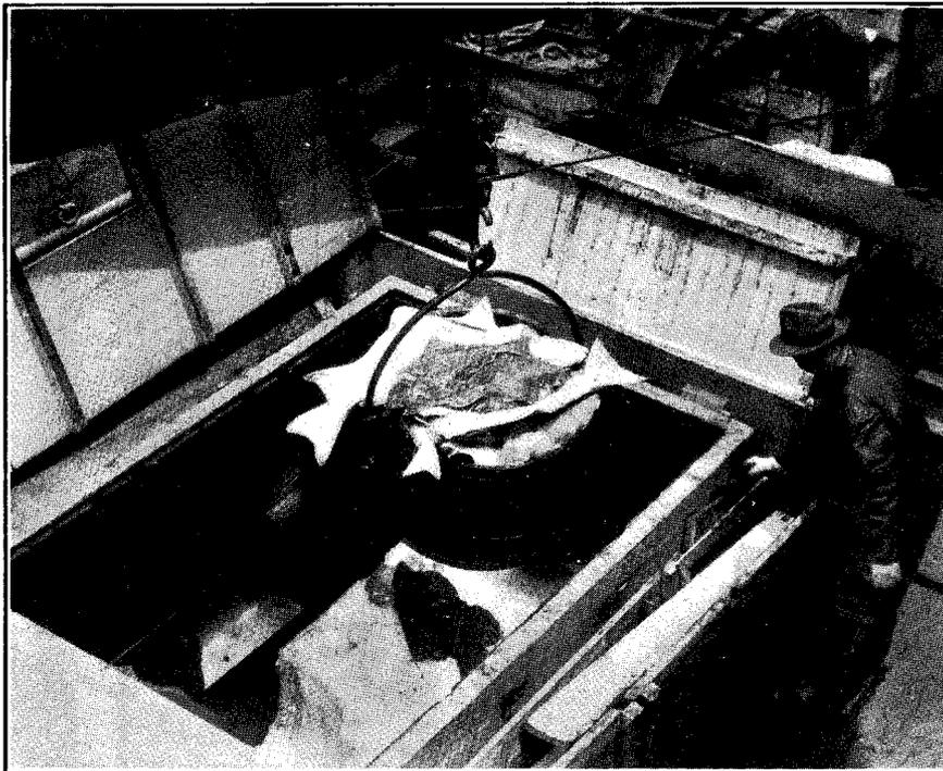
FIGURE 13.—A bucket of fish from the hold. The latter is divided by bulwarks to prevent the shifting of crushed ice and fish. Photo by Ernest Pegler.
