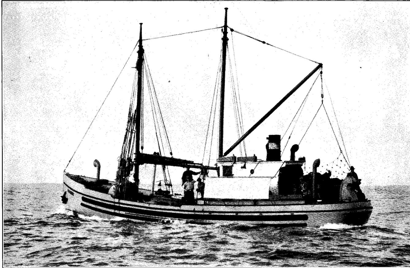
FIGURE 26.—The "Marmot," built in 1926. A modern Diesel-powered long-line boat. Her dories are not for fishing. Note the electric lights, power gurdy, canvas shelter for bait tables, and chute on the stern. The sail is almost lacking.
