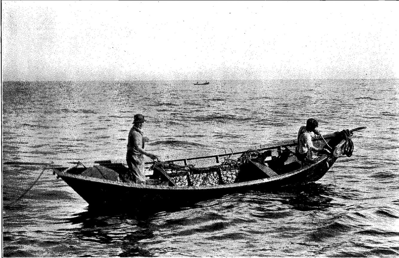
FIGURE 16.—A dory at work. The line is taken in over the gurdy, the fish thrown in the landing net, and the gear coiled in front of the standing fisherman.
