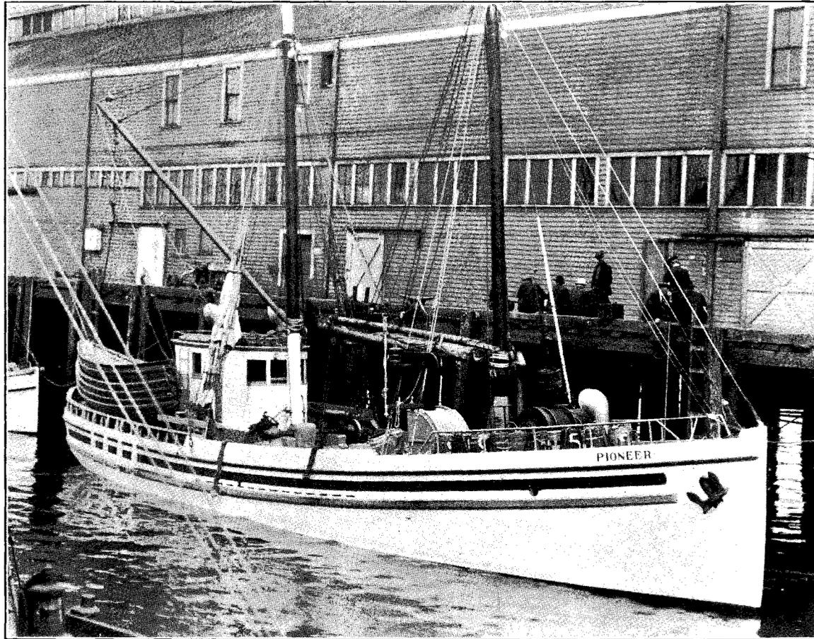
FIGURE 25.—A Diesel-powered dory vessel of a type still in use. Built in 1914. The dories are nested on the stern, there is a gurdy amidships, and a steel anchor cable and winch forward.
