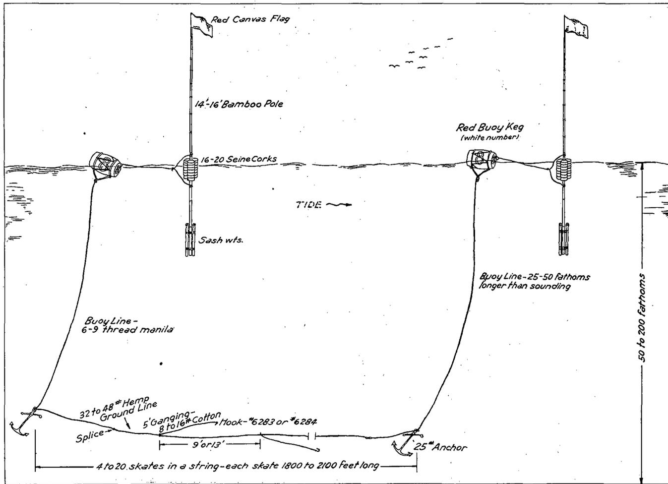
FIGURE 10.—Diagram of halibut gear as set.
