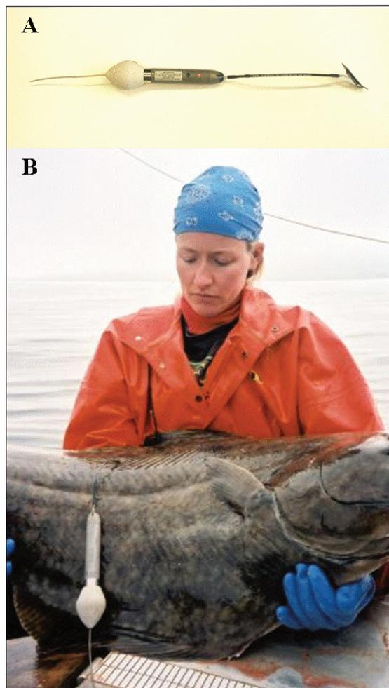
**Figure 1. Pop-up Archival Transmitting (PAT) tags. A) The tag attached to the tagging leader, prior to deployment. The tag's antenna is on the left, and the leader and dart extend to the right. B) A tagged halibut ready for release (*lower photo credit: Lynn Mattes, ADF&G*).**
